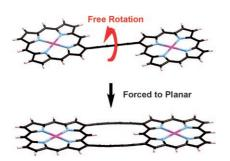
Plane and simple! Doubly  $\beta$ -to- $\beta$  1,3butadiyne-bridged diporphyrins have been synthesized efficiently through metal-catalyzed reactions. The double bridges enforce the two porphyrins in a perfectly planar conformation (see picture), which leads to almost a 100% increase in the two-photon absorption cross section.
