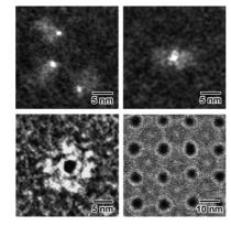
Tag it: Well-defined monomers, dimers, trimers, three-dimensional spherical shells, and two-dimensional ordered arrays of genetically engineered proteins were constructed by using functionalized gold nanoparticles. Nanoparticle size, functionality, and protein genetic motif contribute to the unique geometry, precise stoichiometry, given orientation, and high specificity of these nanoparticle—protein hybrid structures.
