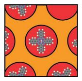
A nanotemplate surface that functions as a regular array of traps for molecules such as naphthalocyanine (see picture) is provided by a nanomesh of hexagonal BN on Rh(111), which has now been identified as a single, complete monolayer. The 2-nmsized pores form at regions where the layer binds strongly to the underlying metal, while the regular network of mesh wires corresponds to regions where the layer is not bonded to the substrate.
