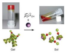
No backbone required: A supramolecular hydrogel has been synthesized from a guest-modified cyclodextrin (CD) without a polymer backbone. The  $\beta$ -CD forms supramolecular fibrils through host-guest interactions, and then hydrogen bonds between the CDs cross-link the fibrils to give a hydrogel. Gel-to-sol transitions can be effected by adding a competitive guest or a denaturing reagent (see example).
